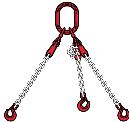
With multi-link assembly, shortening clutches and sling hooks
