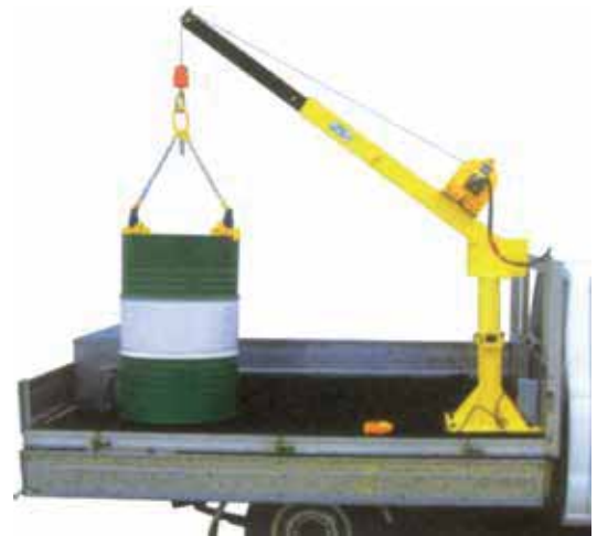
Application Example: My-T-Lift with manual brake winch mounted on truck cargo area.
