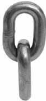
Grade 80 – 16mm WLL 8.0t 1 Metre = 5.65kg
