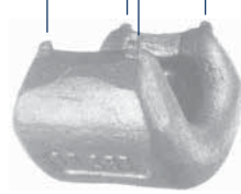
Distance lugs for root weld.
