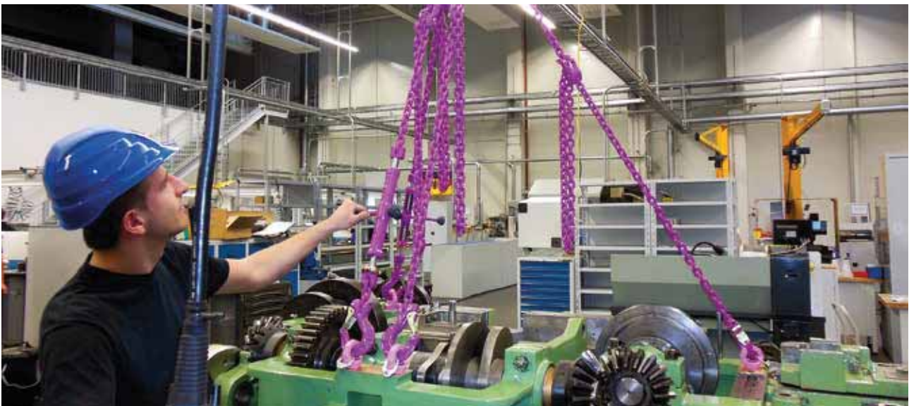
ICE 120 – 13mm WLL 8.0t 1 Metre = 4.25kg
